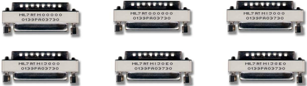
Figure 6: MIL run-time hardware license keys (dongles), shown only for the parallel port, are available for various MIL run-time packages. The stamp identifies which package the dongle is valid for (e.g., dongle labeled 'MIL 7 RT 0 0 0 G 0 0' is valid for the GMF module).
