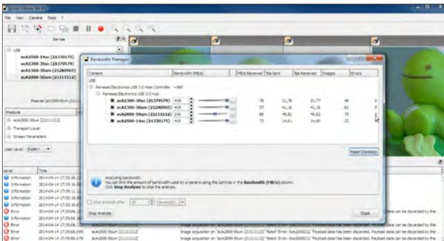
With the viewer's new Bandwidth Manager you can quickly check whether your USB3 or GigE camera can reliably deliver all images to your application (e.g. the pylon Viewer) with the given bandwidth settings. You can adjust the camera's bandwidth load until all cameras connected to your PC will transmit their images without any losses.
