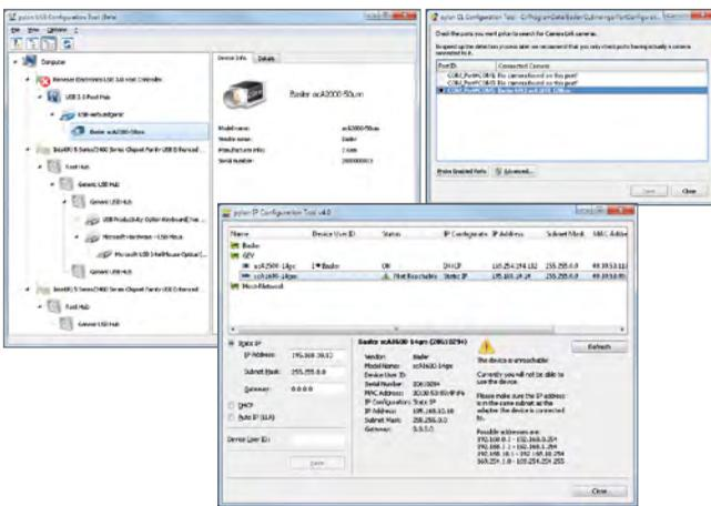
For example, you can easily configure the IP settings of a GigE Vision camera, fix driver or bandwidth problems for USB cameras, or configure baud rates for Camera Link cameras.
