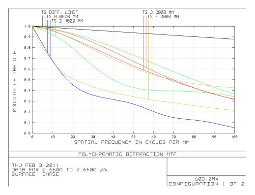
Working distance: 400mm F-stop: 1.4 Wave length:  $\lambda$  =660nm\_mono
