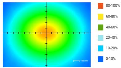
Optical measurement taken using LL17406-WHIIC Rev. A @ 300mm
