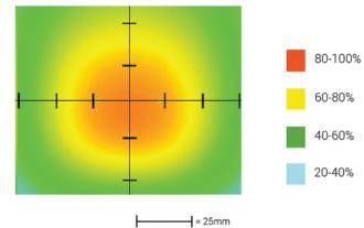
Optical measurement taken using DL225-150WHIIC @ 25 mm
