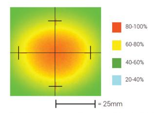
Optical measurement taken using DL225-025WHIIC @ 25 mm
