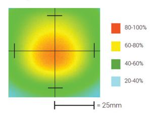
Optical measurement taken using DL225-050WHIIC @ 25 mm
