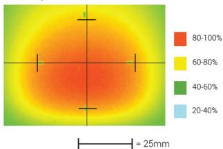
Optical measurement taken using DL225-100WHIIC @ 25 mm
