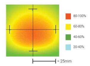
Optical measurement taken using DL225-075WHIIC @ 25 mm
