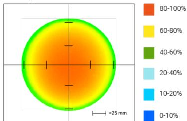
Optical measurement taken using DL097-WHIIC Rev. A @ 25 mm
