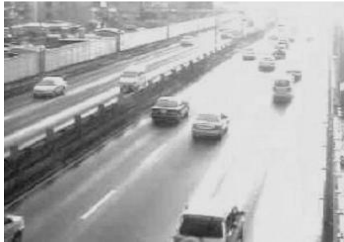
Figure 5. A typical traffic surveillance video recorded image. The huge intra scene dynamic range is created by the Sunset, but not by the objects in the scene.
