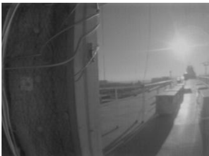
Figure 6. A sample image from a MAGIC camera chip of a scene with huge intra scene dynamic range. The MAGIC camera chip produces a very pleasant image conserving the visual detail over the whole scene in this extreme lighting conditions.
