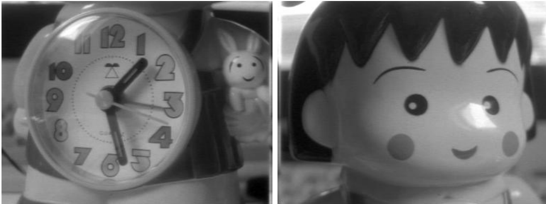
Figure 13. By placing the logarithmic image in an adequate interval, a very pleasant \gamma=0.5 image can be obtained. The images have been captured from a 352x288 MAGIC camera chip designed and fabricated in AMS 0.35um CMOS. Please note that the images are coded only in 7-bit despite of the large dynamic range of the scene due to the presence of specular reflections.
