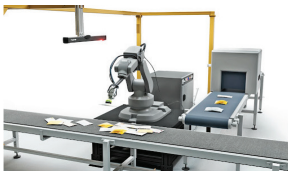
Picking from conveyor
