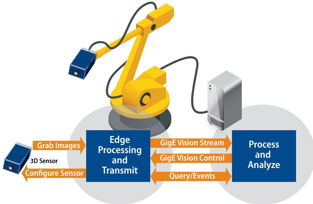
*Software techniques enable the design of “virtual GigE Vision” sensors that can be networked to share data with other devices as well as local and cloud-based processing.*
