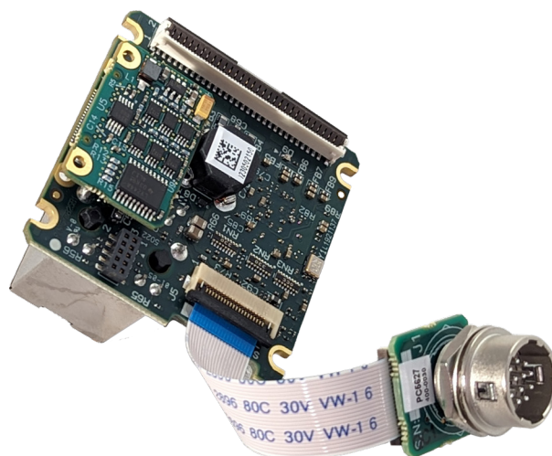
iPORT NTx-Mini Embedded Video Interface main board with horizontal RJ-45 connector and soldered 12-pin circular connector on the FlexEBoard
