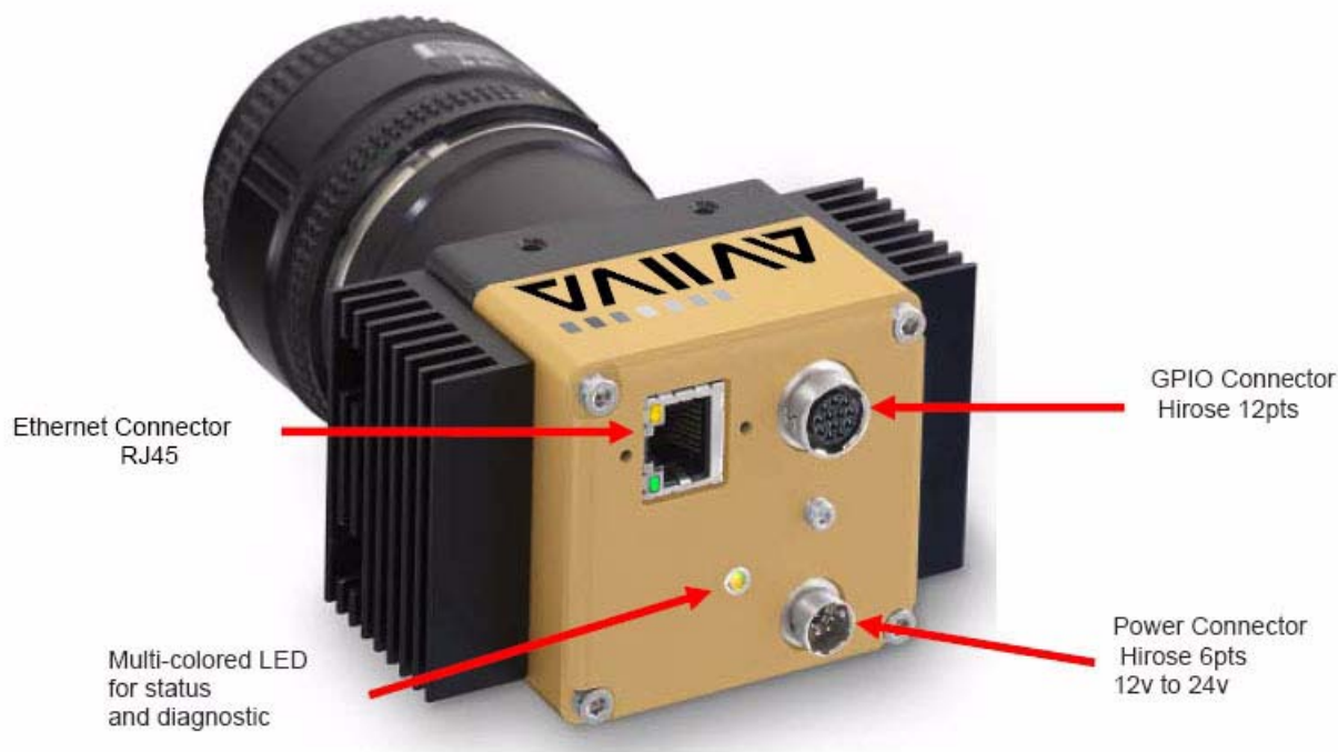
Figure 4-3. Connectors and LED
